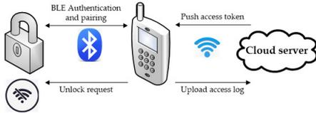
Figure 1: DGC model of smart lock
